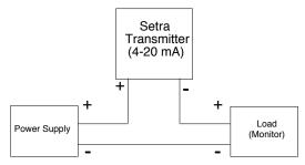
The 4-20mA current output circuit is designed to have current flow in one direction only **please observe polarity**. It is suggested that the cable shield be connected to the system loop circuit ground to improve electrical noise rejection.
