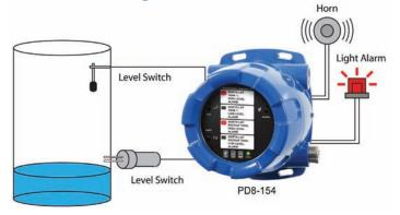
The ProtEX-MAX Annunciator is ideal for tank level switch monitoring.
