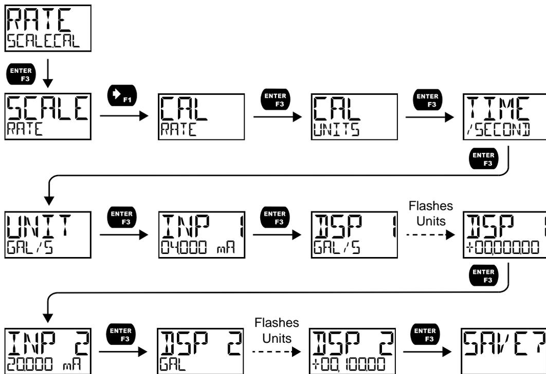
1. After accessing the SCALECAL menu, press the **Right-Arrow** button to scroll to the *Calibration* menu (CAL RATE) and press *Enter*.
