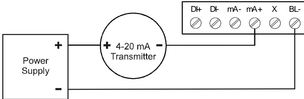
Figure 6. 4-20 mA Input Connection with Backlight
