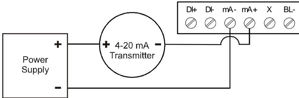
Figure 5. 4-20 mA Input Connection without Backlight
