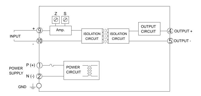
\* A short circuit between the output terminals (#4 and #5) must be avoided as it may cause a failure.
