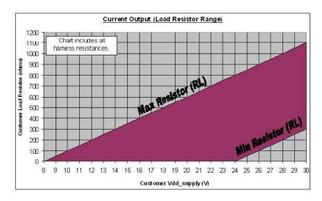
$\label{eq:min-selector} \begin{array}{l} \mbox{Min Resistor (RL)} = 50 * (Vdd\_supply - 24) : \mbox{for Vdd} > 24V \\ \mbox{Max Resistor (RL)} = 50 * (Vdd\_supply - 8) : \mbox{for Vdd} > 8V \\ \end{array}$
