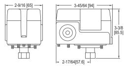
The **Series CXA Water Pump Pressure Switch** has been proven reliable for controlling automatic water systems. These switches are very popular for use on water well pumps and pumping systems. The set point and dead-band are both easily adjustable via screws inside the cover. For ease of installation, the switches come with a 1/4" female NPT process connection and can be mounted in any orientation. The series CXA's simple design makes it a great switch for an installer at any skill level.
