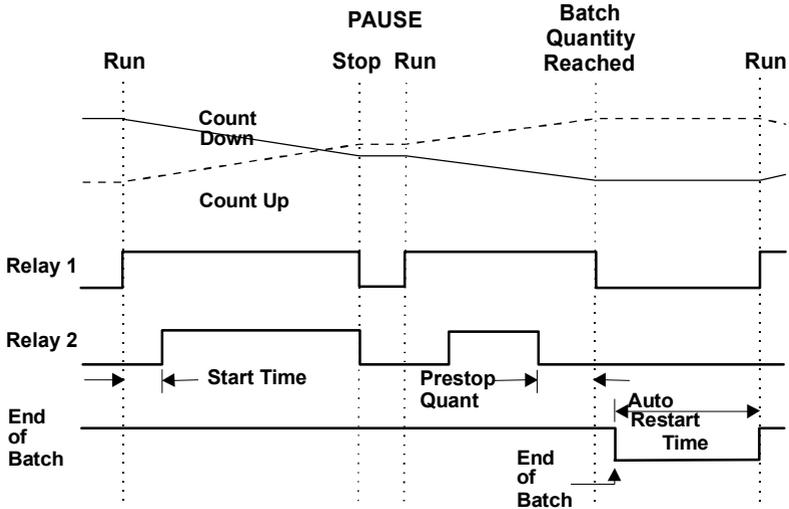
The Batch Controller can also be programmed, during Calibration, to either count up from zero on each batch, or to count down from the preset batch quantity.
