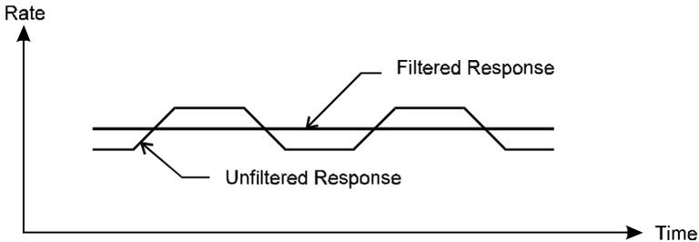
As a guideline to the degree of filtering to be used, the following table shows the response to a step change in input. The value, A, is the filter constant which is programmed during the Calibration routine. The times for the display value to reach 90% and 99% of full swing are given in seconds, for different values of A.
